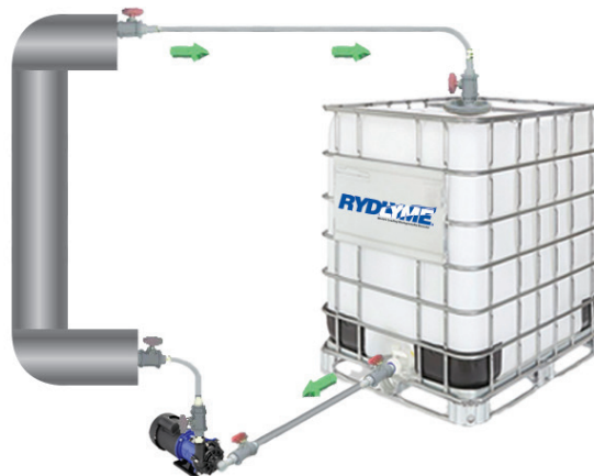
Circulation set up for cleaning pipeline with RYDLYME . Visit our website for available pumping systems!
